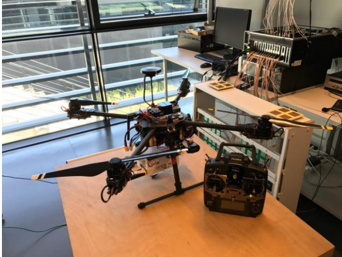
Figure 1 Photo our our robot prototype, carrying a fully functional 4G base station.
